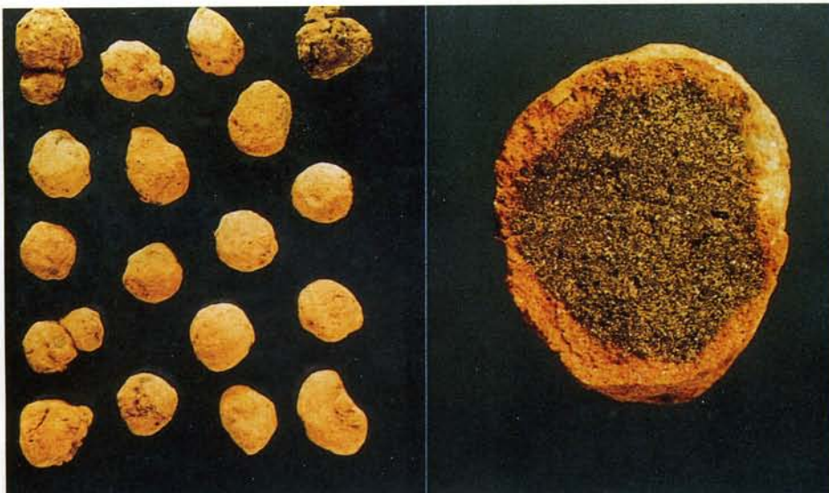
Lytag particles and cross-section. This sintered pfa product has an open interior with a glassy outer skin
