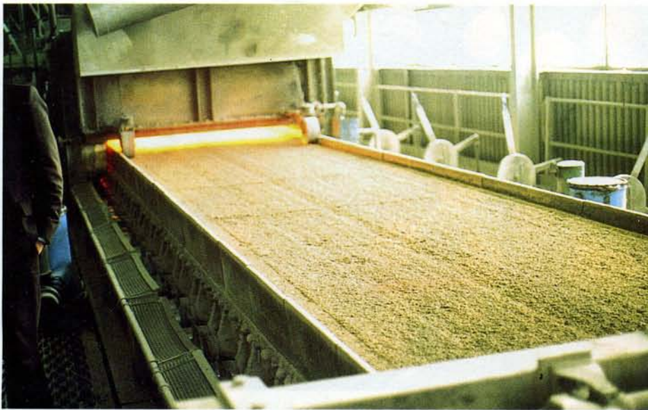
Sinter strand for the production of Lytag with ignition hood in the background
