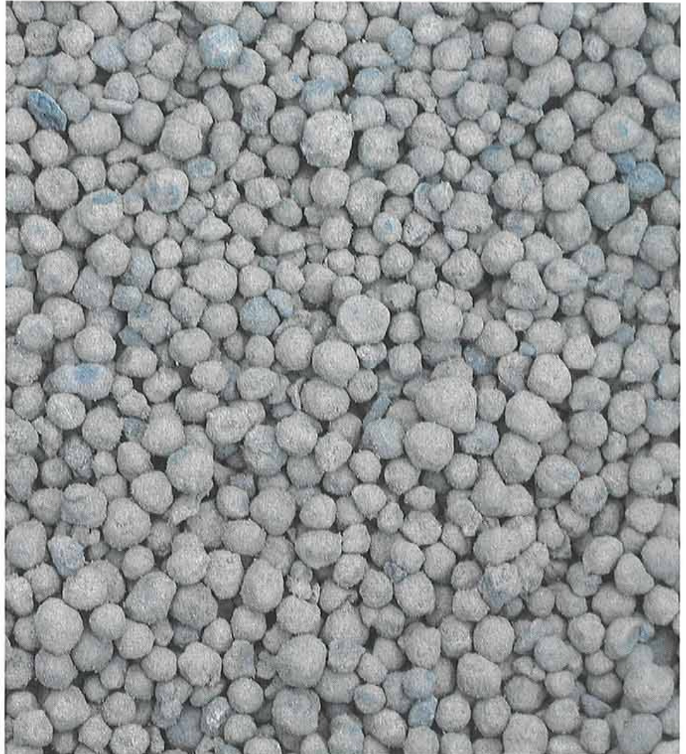
Lytag lightweight aggregate provides significant weight savings in concrete
